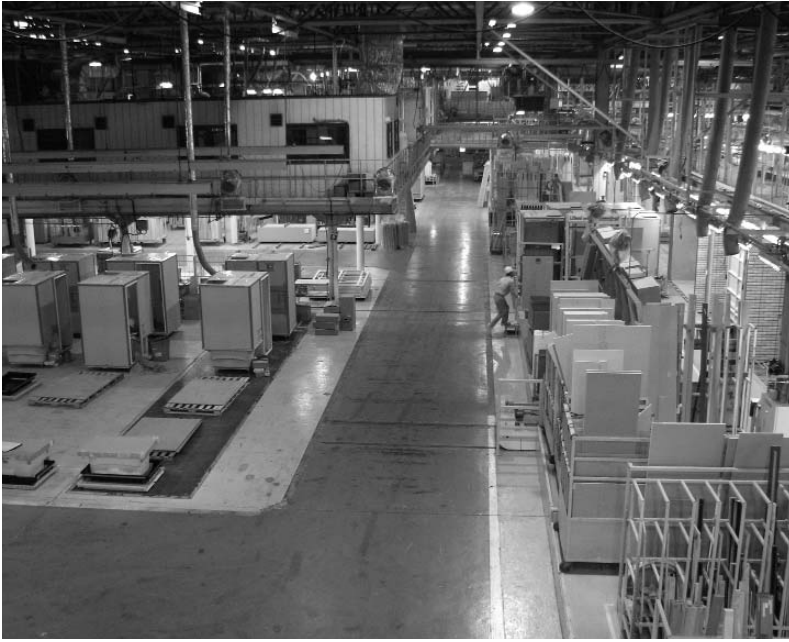
Figure 3. About two hours of line side inventory is at the right. With such big items, material movement is highly visible in this plant. At left, about a half day's production of bathroom modules are waiting to be trucked to their building sites. Most bathrooms are small by American standards.
