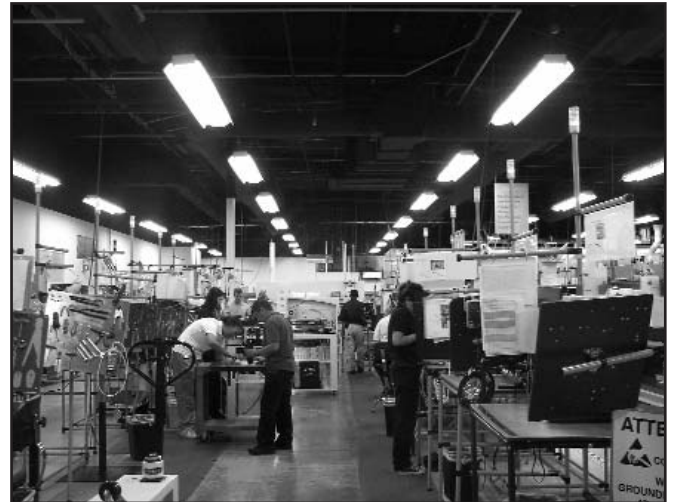
Figure 5. At right, a view of the BenchMark XT sub-assembly as it was being created using mock ups. At left, the BenchMark XT cell as it appears today, many kaizens later, feeding final assembly and test, which can be seen in the far background. Note the hanging shadow boards for tools, the hanging work instructions, and an andon for each station. Andon lights are called "And On" lights in Ventana.
