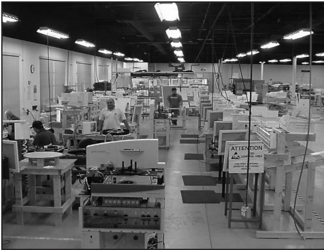
Figure 5. At right, a view of the BenchMark XT sub-assembly as it was being created using mock ups. At left, the BenchMark XT cell as it appears today, many kaizens later, feeding final assembly and test, which can be seen in the far background. Note the hanging shadow boards for tools, the hanging work instructions, and an andon for each station. Andon lights are called "And On" lights in Ventana.
